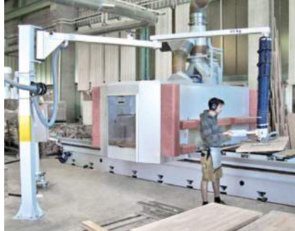
Articulated-arm jib to move around obstacles
