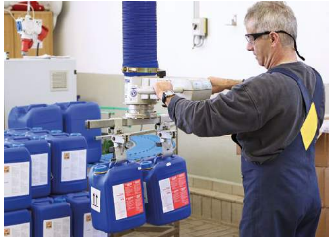
Vacuum tube lifter JumboErgo with mechanical gripper for handling jugs
