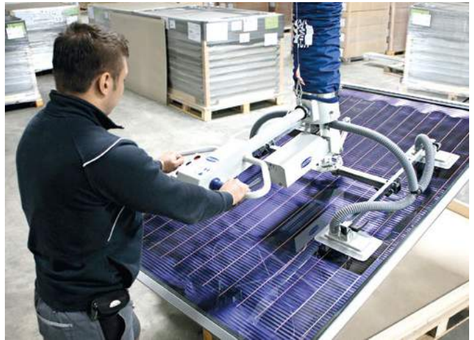
Solar | Vacuum tube lifter JumboErgo with 90° swivel angle for handling solar panels
