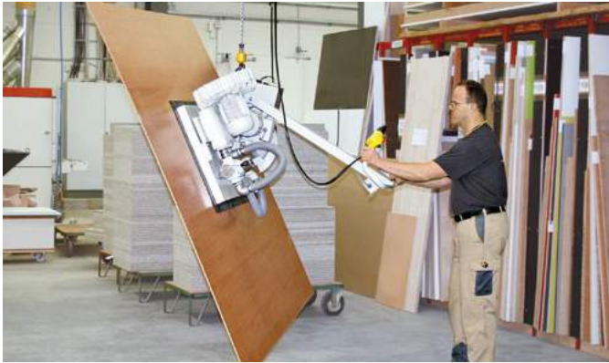
VacuMaster Multi for swiveling wooden boards by 90°
