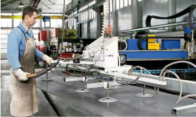
VacuMaster Vario in process of loading and unloading a laser cutting machine
