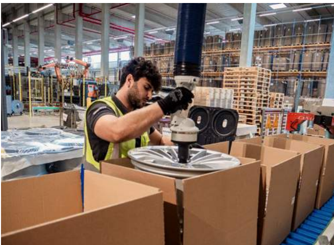
Vacuum tube lifter JumboFlex with pneumatic mandrel gripper for handling wheel rims
