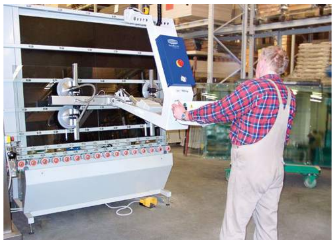
VacuMaster Comfort for turning a glass sheet by 180°
