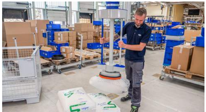
Jumbo Low-Stack when handling bags
