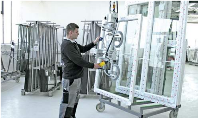
VacuMaster Window for rotating and palletizing windows
