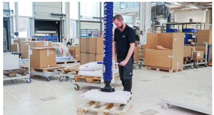
JumboFlex High-Stack when handling bags
