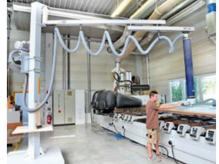
Telescopic jib for confined working areas
