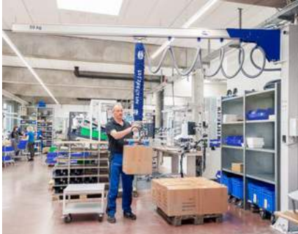
Modular flat jib for particularly low ceilings
