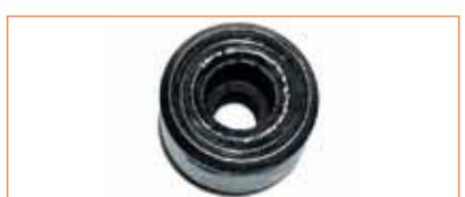
interior ring damaged for 100%
