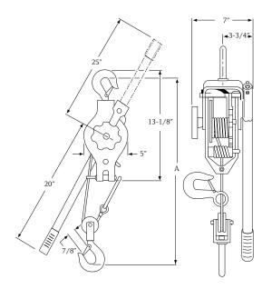
Overload safety handle is designed to bend — when an overload is detected. Once the handle begins to bend, additional force will limit the hoist from lifting beyond its capacity.
