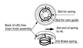
Set (43) Brake spring (silver color) into the slot of the back of (45) Free chain knob assembly.
