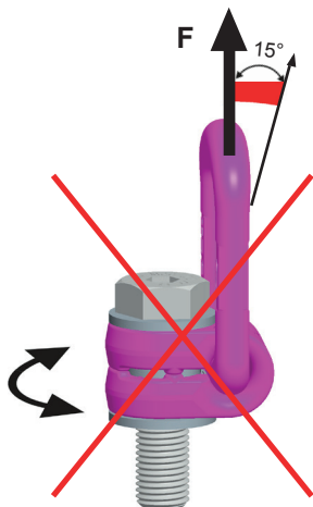
Pic. 7: Forbidden turning direction at loading in the direction of the axle.
