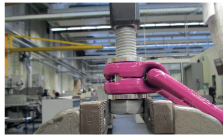
Pic. 8: Dismantling position of the VLBG
